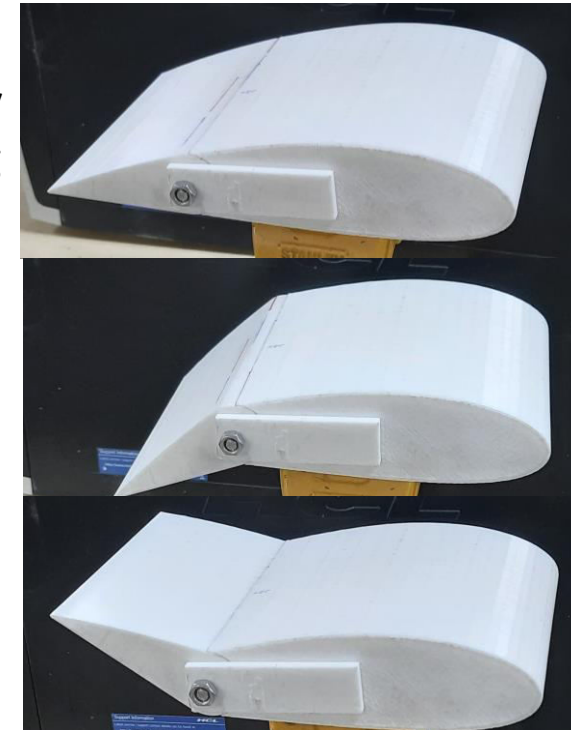
Fig. 2 Prototype of the morphing aerofoil
